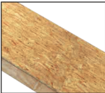
Roof deck (OSB)
